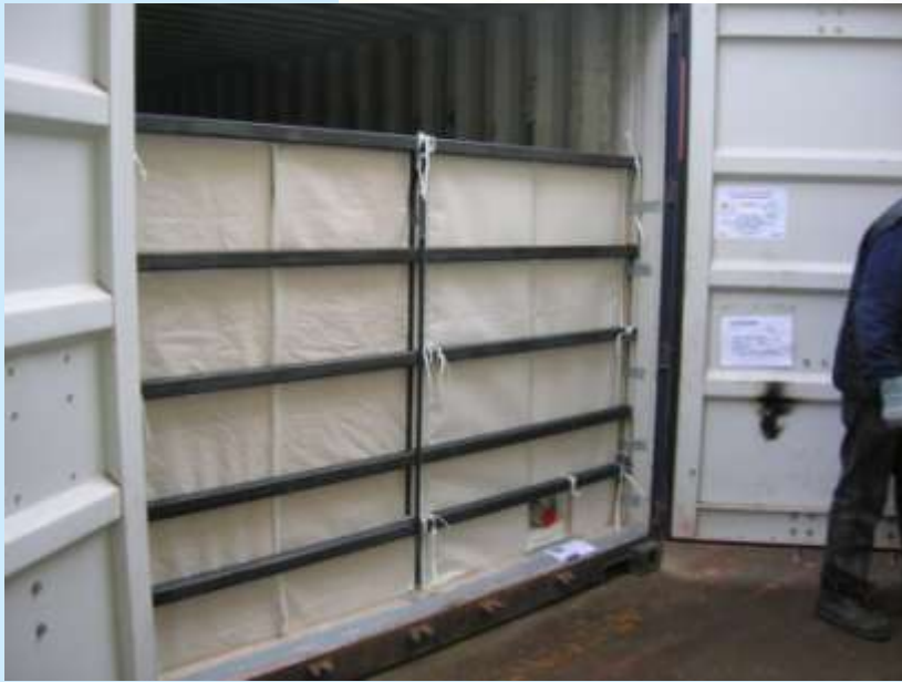
Bulkhead installation – bottom valve
